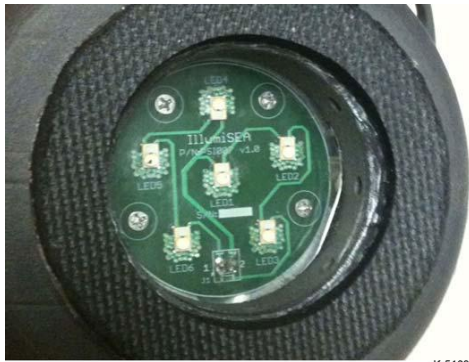
Figure 2. View into the flow chamber showing the six LEDs mounted on the custom circuit board
